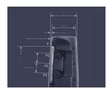
Diameter, Chamfer Lead, Taper, Distance at Single Cutting Edge Reamers
