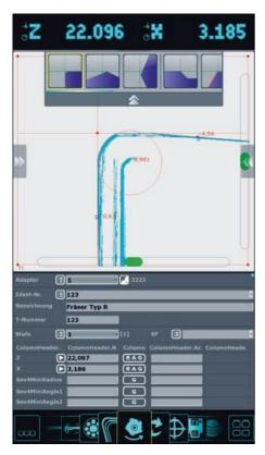
Software function for determining and measuring the maximum contour of all the cutting edges of a tool.
