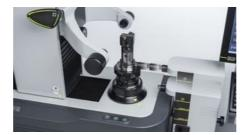
Automatic tool identification The read/write head is moved fully automatically using CNC axes to the RFID chip on the tool holder clamped in the ZOLLER presetting and measuring machine. The tool data is written automatically by the RFID system to a code carrier on the tool holder and can be read at the processing machine.
