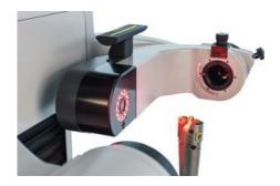
Tool inspection For axial and radial inspection and testing of the contours of radii, angles, distances and wear and tear in incident light, with 50-times magnification of the cutting tool edge.
