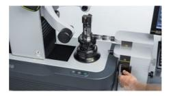
Semi-automatic tool identification The read/write unit is moved manually in the Z direction at the height of the RFID chip on the tool holder. The read/write head is moved in the X axis by the CNC controls. When the read/write unit detects the RDIF chip, it can be read and written to.
