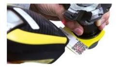
»zidCode« with labels With »zidCode«, data is quickly and easily printed onto labels and can be scanned directly into the CNC machine control. This means data transmission without errors.
