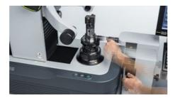
Manual tool identification The read/write head is moved manually over the RFID chip on the tool holder. This chip can then be read and written to.
